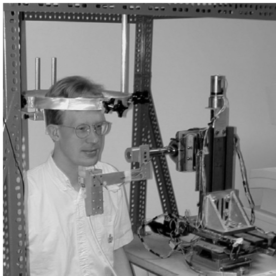
Figure 3D. Head and Transducer Support (HATS) system uses a rigid transducer position and acoustic standoff.
